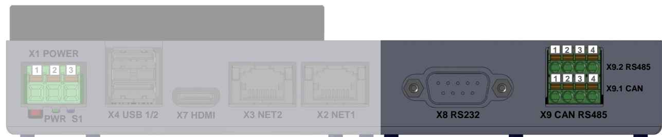
Figure 4: Interfaces/Connectors Extension part Front side of the model CU 5x-2x1x
